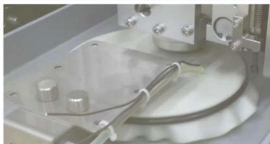
One-piece-flow automatic-sliding plating machine
