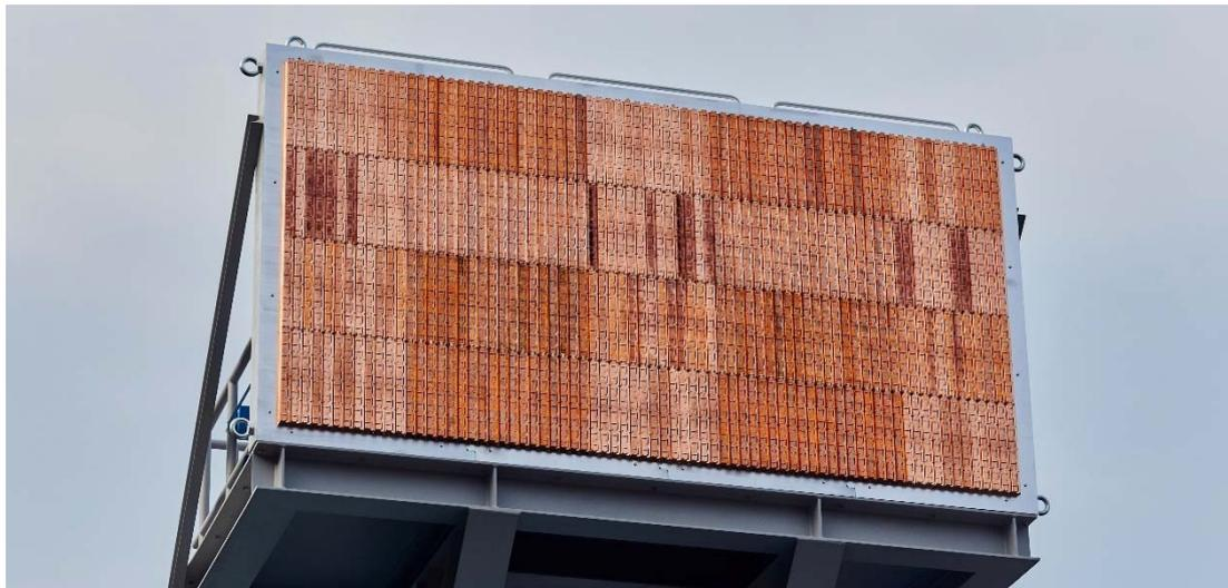
Prototype of resin-injection-molded waveguide array antenna
